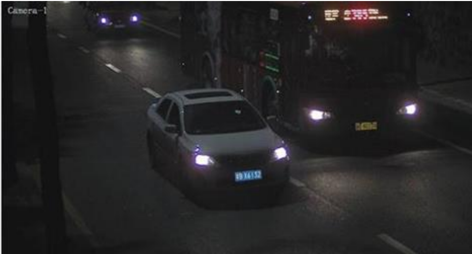
Figure 13a: License plate contrasts at 10m from a passing vehicle. The IR source is located at 5m from the video camera
