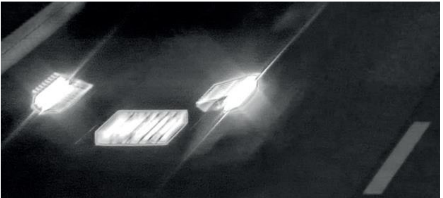
Figure 20: A car moving at high speed is imaged with an exposure time of 1/30 s
