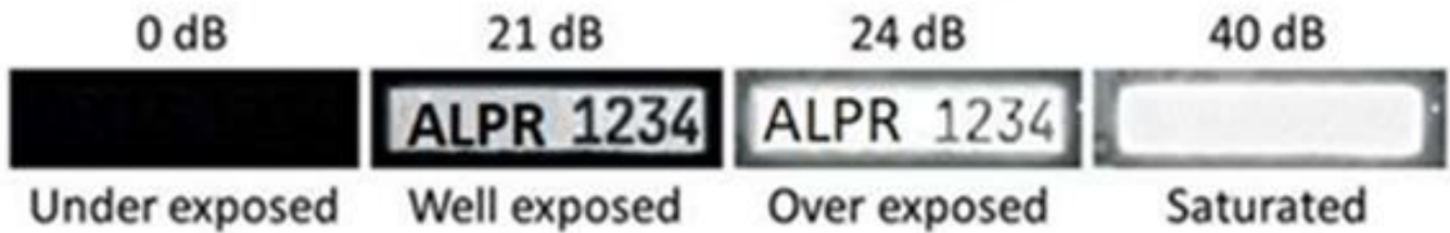
Figure 21: The max gain setting will determine how the license plate is exposed at night
