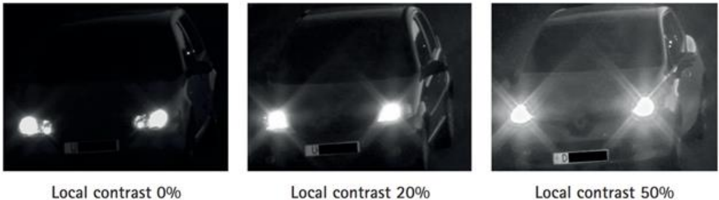
Figure 22: Local contrast on a camera with ARTPEC-6 is a tradeoff between good contrast in the license plate, and too much noise and glare in the image
