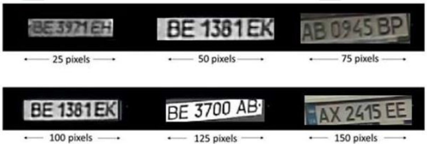
Figure 5: A European standard license plate should cover at least 75 pixels for the letters to be imaged with full contrast. Most LPR software requires 100-150 pixels over the width of the plate
