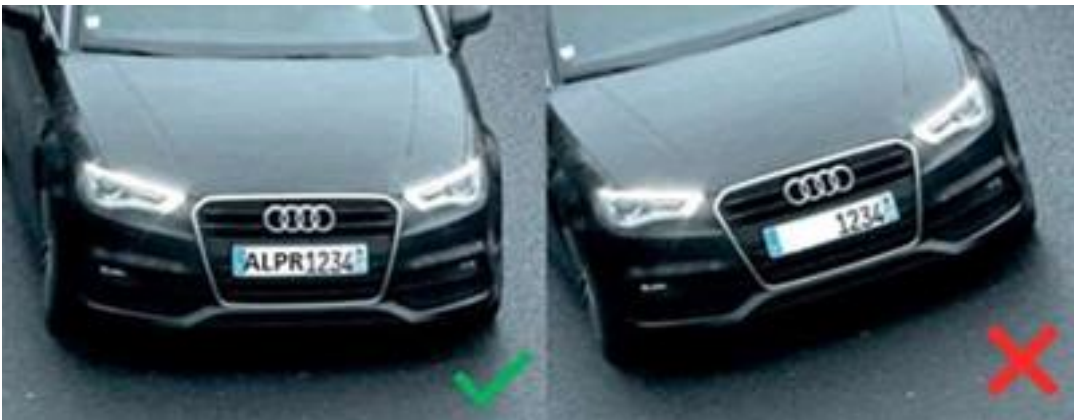
Figure 16: The camera should be aligned so that the license plate is parallel to the edge of the image
